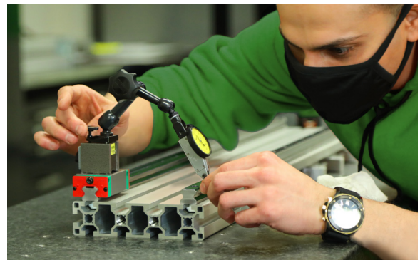
Fig. 2 Ensuring parallelism of the master rail and subsidiary rail
