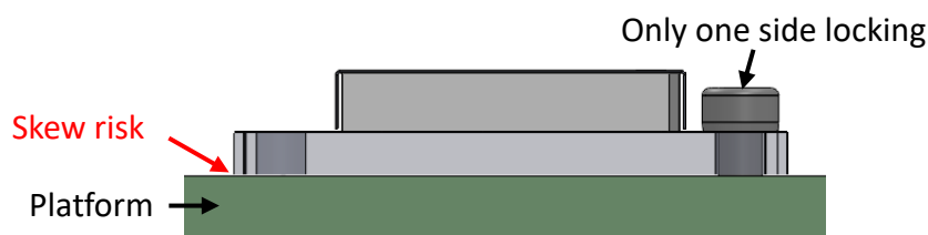
Figure 4.1.1.2.11 Avoid skewing after tightening the unilateral screws
